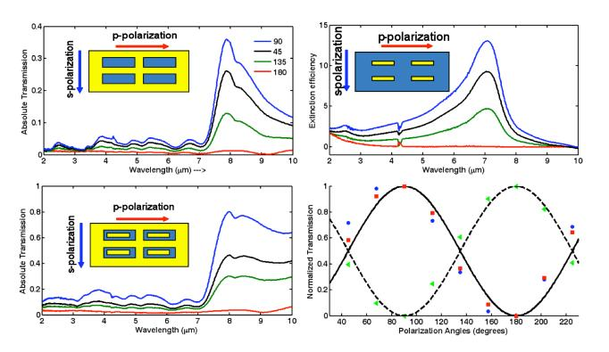
Yanik et al (2009) Polarization dependence of the EOT signal is shown for (a) rectangular and (b) coaxial nano-cavities. Extinction efficiency for Nanorod antennae is given for changing polarization angles for incident light. (d) Complementary behavior of cavities and nanorod is observed.
