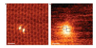
"Atomically localized plasmon enhancement in graphene" Zhou et al Nature (2012) EELS (Electron energy loss spectroscopy)
