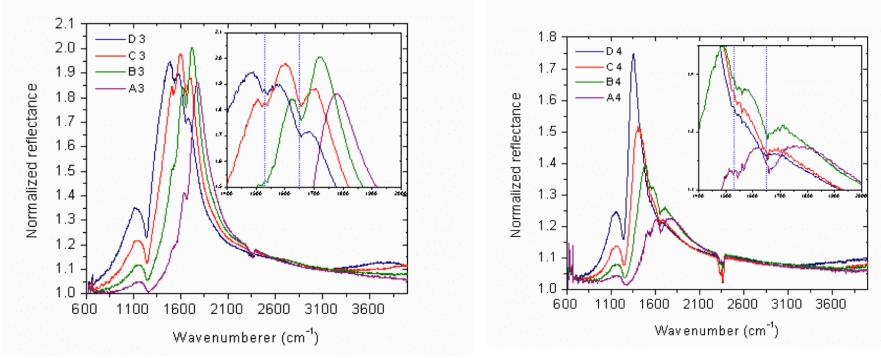
Rows 3 and 4 of chip 1213c (left, right) correspond to periodicities of 1.5 and 2  $\mu$ m respectively, with rods 200 nm in width. Inset: Blue lines 1530 and 1650 cm<sup>-1</sup> [Adato et al; with Amsden, Kaplan, Omenetto, Tufts]
